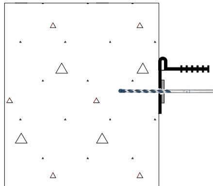
5) Using the prepunched stainless steel batten bar as a template, drill 1/4" holes 2-3/4" deep through waterstop and concrete. Clean out holes. can.
