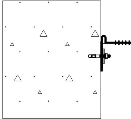
10) Hammer stainless steel wedge anchors into drilled holes, passing anchor through batten bar, waterstop and epoxy gel bed. Repeat for all holes. Tighten anchor bolts.
