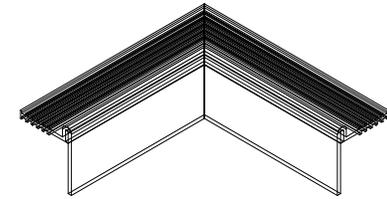
3) Heat weld waterstop profile to appropriate length and directional changes to fit concrete surface.
