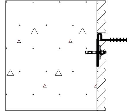
11) If expansion joint install expansion joint filler above and beneath waterstop embedment leg.
